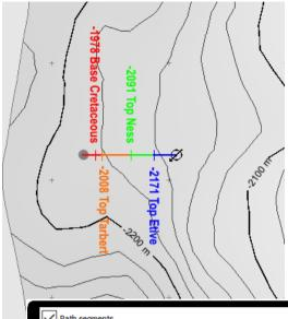
Displaying well path segments helps visually identify and highlight the spatial distribution of key producing zones, sands or reservoir properties.
