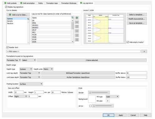
A new Log signature, tab is available under the /Display/Wells option in mapping. This provides users with a range of focused display style, annotation and controls.
