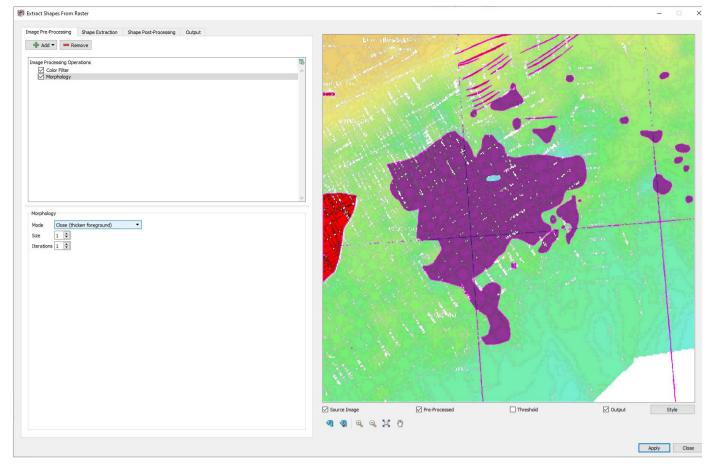
Image processing is applied to remove the seismic lines, faults on the map image (shown above). Then the users highlights the polygons from the image – shown below in the threshold bitmap view (black and white). These resulting polygons are extracted and can be saved to a variety of file formats supported by our spatial data outputs, eg shapefiles, geodatabases, 3<sup>rd</sup> party data sources, etc.
