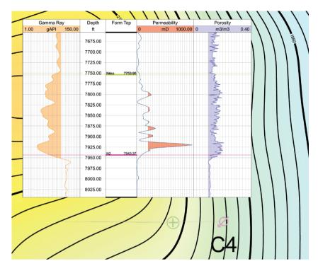
Logs display can be limited by depth or markers recorded for the borehole.
