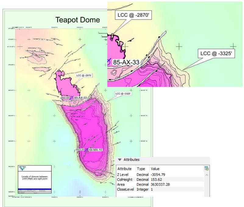
The output can be mapped using the **Display/GIS** option including posting, filtering and thematically mapping by attribute.
